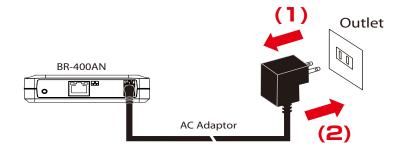
**2.** When the POWER LED turns green and WLAN LED turns or blinks green/orange, the restart is completed. After the restart, the BR-400AN will start in a normal mode.
