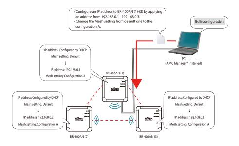
For AMC Manager<sup>®</sup>, there are a free version "AMC Manager<sup>®</sup> Free" and a non-free version "AMC Manager<sup>®</sup>". When a non-free version is used, more devices can be managed and configured at once and the plug-in utilities such as Mesh Monitor, etc. can be used.
