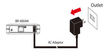
2. Press and hold the push switch on the front (1) while inserting the AC adaptor back into the electrical outlet (2).
