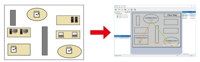
As shown in the image above, the actual installation environment is simulated on Mesh Monitor. The route information is displayed based on the actual route setting of BR-400AN. It is possible to change some functions of BR-400AN using Mesh Monitor (e.g. enabling/ disabling Access Point function, etc.). Also, a history of Mesh network route and BR-400AN's operating status can be checked and which can be used conveniently for troubleshooting.
