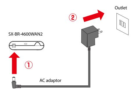
**3.** When the POWER LED on top of SX-BR-4600WAN2 turns on, press and hold the push switch on the front. Release the push switch when the WLAN LED and STATUS LED start blinking together (it may take 20sec until blinking). SX-BR-4600WAN2 will start operating in the Configuration Mode and you will be ready to configure SX-BR-4600WAN2 from the PC.
