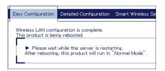
When you wish to bridge the PC used for this configuration wirelessly, restart the PC. To bridge another device wirelessly, turn off both SX-BR-4600WAN2 and PC, remove the SX-BR-4600WAN2 from the PC and connect the SX-BR-4600WAN2 to the device you wish to use wirelessly using a network cable. For details, refer to **Connecting Non-wireless Devices** in the next page.
