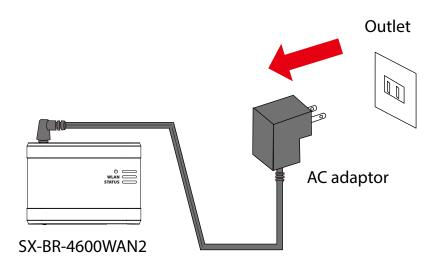
**2.** Press and hold the push switch on the front while inserting the AC adaptor back into the electrical outlet.
