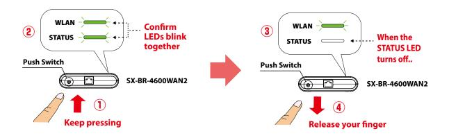
**6.** The SX-BR-4600WAN2 and the Access Point will start to communicate each other. When the configuration finished successfully, the STATUS LED turns on or blinks.
