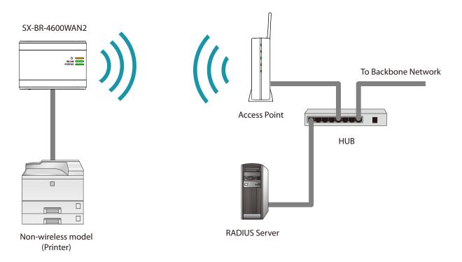
When using the authentication method that requires a certificate, get the necessary certificate issued by the certificate authority and import it to the SX-BR-4600WAN2. To use this function, register the MAC address of non-wireless device with SX-BR-4600WAN2. The reliability of non-wireless devices connected to SX-BR-4600WAN2 is identified using the MAC address filtering.
