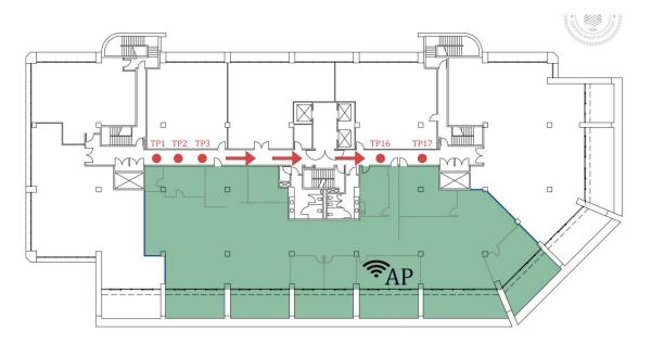
Figure 1: Second floor of the Silex office building; red arrows demonstrate the location of test points, and AP abbreviation identifies each access point location.
