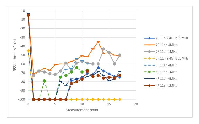
Figure 3: Received signal strength indicator (RSSI) shows wireless wireless signal strength according to the receiver; higher RSSI indicates better signal.
